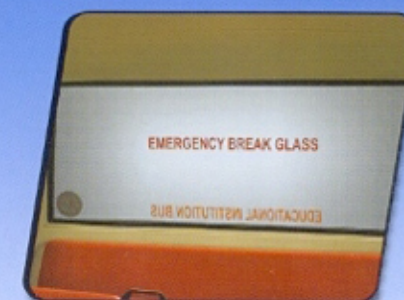
Large emergency exit window
